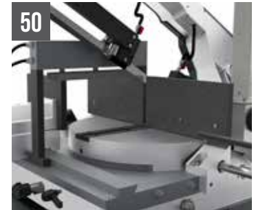
50 SHARK 332-1 SXI evo - Hydraulic overhead bundling for bundle cutting (max 320x160 mm)
