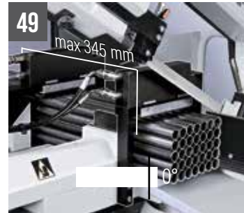
49 SHARK 281 NC 5.0/282 SXI evo Hydraulic vertical vices for bundle cutting (max 170x130 mm)
