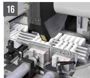
TIGER 402 CNC HR 4.0 set off comb jaws in teflon for bundle cutting (max mm 75x75)
