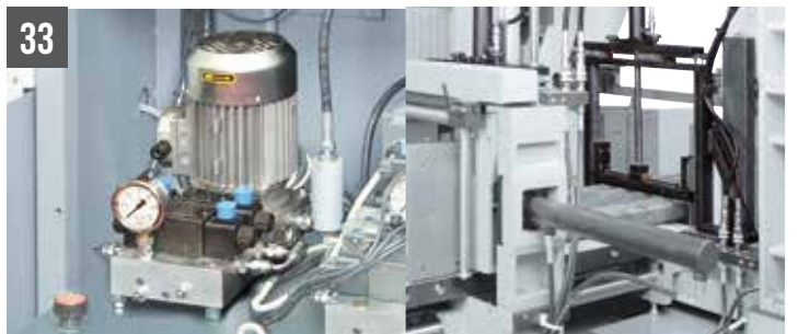
SHARK 350 CNC HS 4.0 - SHARK 460 KONNECT Hydraulic vertical vices for bundle cutting
