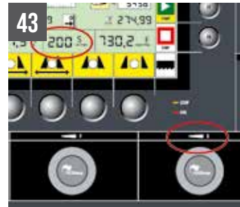
43 SHARK 350 CNC HS 4.0 SHARK 350 NC HS 5.0 Kit cutting speed 15÷200 m/min
