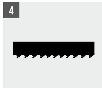
Band with electowelded hard metal plates
