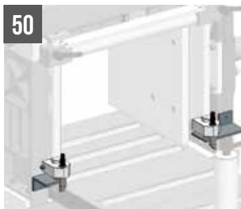
50 Shark 350 CNC hs 4.0 Bar sensor to optimize restpiece (3 special cutting cycle)
